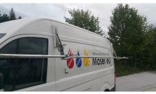
Even smaller people can work with it, simply fold it out and load it. The holder also offers an ecological advantage, since this causes less air resistance and noise when not in use in the folded state compared to a roof rack. It can carry loads up to 150kg.
